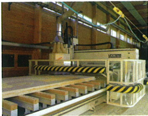
LEFT: A panel being CNC cut and routed in the KLH factory, Austria.
